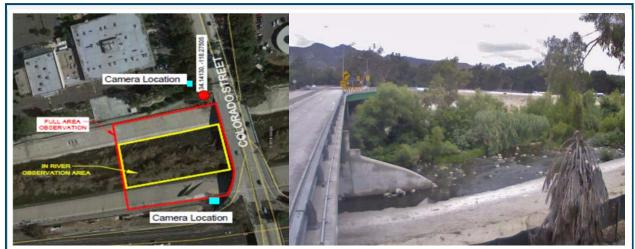
Figure 12: A typical continuous monitoring location aerial view showing camera installations (left) and a typical camera vantage point (right).
