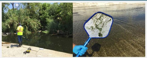
Figure 11: A typical seining measurement using a net with the flow velocity equipment shown in the foreground (left) and a typical result of the seining measurement showing no trash present (right).
